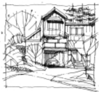
Minimize the impact of the car by placing garages under buildings or decks above
