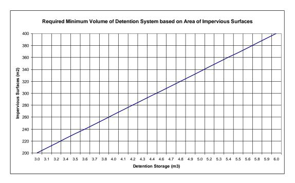
2. Any connection from a stormwater detention system to the municipal storm drainage system shall have a restricted outlet, sized according to the following table. The system may also have an overflow connection, located at the highest point possible to ensure the system detains its full capacity.
